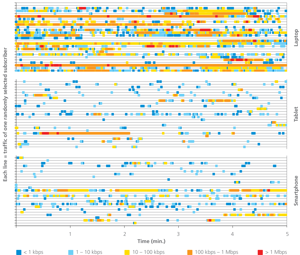
Figure 28: Data transmission patterns from laptops, tablets, and smartphones as examined over a five-minute period
